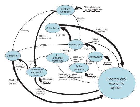
**Figure 4** Selected industrial symbioses in Lubei Industrial Park. The variation in the thickness of the lines is an indication of the magnitude of the flows; the squiggly lines indicate the raw materials taken from nature outside the eco-industrial parks.  $SO_2$  = sulfur dioxide; kt = kilotonne; kwh = kilowatt hour; NaOH = sodium hydroxide.
