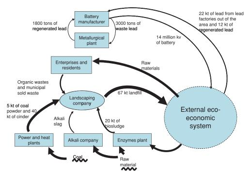
**Figure 6** Selected material flows in the industrial symbiosis in the Tianjin Economic Development Area. The variation in the thickness of the lines is an indication of the magnitude of the flows; the squiggly lines indicate the raw materials taken from nature outside the eco-industrial parks. kt = kilotonnes; kv = kilovolts. Source: Based on the work of Tan and Bao (2006), Geng and Yi (2006), and Shi and colleagues (2010).
