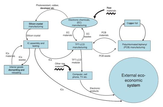
**Figure 5** Selected industrial symbioses in Suzhou Industrial Park. The variation in the thickness of the lines is an indication of the magnitude of the flows; the squiggly lines indicate the raw materials taken from nature outside the eco-industrial parks. IC = integrated circuit; TFT-LCD = thin-film transistor liquid crystal display; PCB = polychlorinated biphenyl.
