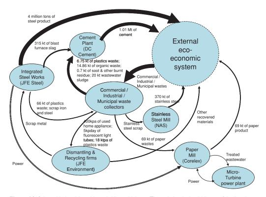
**Figure 10** Selected industrial symbioses in Kawasaki, Japan. The variation in the thickness of the lines is an indication of the magnitude of the flows. Mt = megatonnes; kt = kilotonnes; ktpa = kiloton per annum; kpa = thousands of items per annum; kpd = thousands of items per day. Source: Based on the work of Van Berkel and colleagues (2009).
