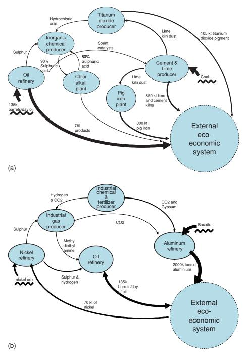
**Figure 8** (A) Selected industrial symbioses in Kwinana, Australia (1) with focus on titanium dioxide. (B) Selected industrial symbioses in Kwinana, Australia (2) with focus on nickel. The variation in the thickness of the lines is an indication of the magnitude of the flows; the squiggly lines indicate the raw materials taken from nature outside the eco-industrial parks. k = k1 klotonnes; k = k2 thousand. Source: Based on the work of Van Beers and colleagues (2007).
