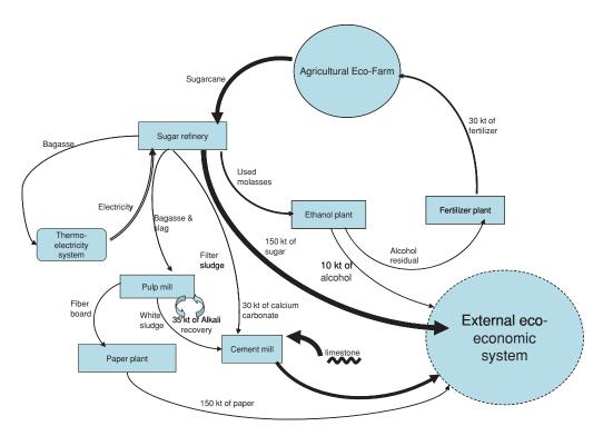
**Figure 2** Selected industrial symbioses in the Guitang Group, Guigang City. The variation in the thickness of the lines is an indication of the magnitude of the flows; the squiggly lines indicate the raw materials taken from nature outside the eco-industrial parks. kt = kilotonne.
