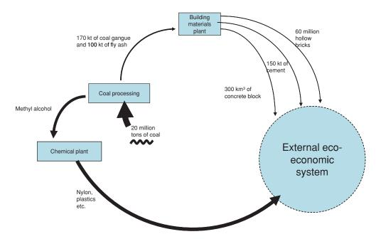
**Figure 3** Selected industrial symbioses in the Pingdingshan Coal Mining Group. The variation in the thickness of the lines is an indication of the magnitude of the flows; the squiggly lines indicate the raw materials taken from nature outside the eco-industrial parks. kt = kilotonne; km = kilometer. Source: Based on the work of Long and Zhang (2009) as well as Pingmei's Web site (www.pmjt.com.cn).
