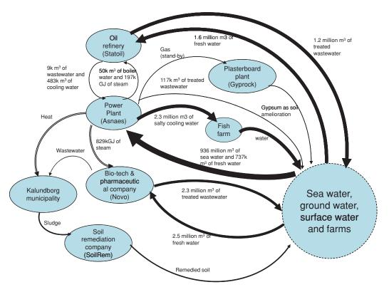
**Figure 7** Selected industrial symbioses in Kalundborg, Denmark. The variation in the thickness of the lines is an indication of the magnitude of the flows. m = meters; k = thousand; GJ = gigajoules;  $CO_2 = carbon dioxide$ .
